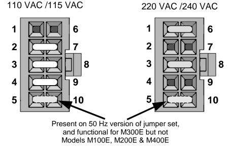
Figure 2-3: Pump AC Power Jumpers (JP7)
